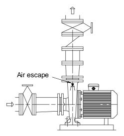
Priming of a flooded pump
